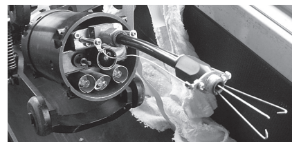
写真6 異物回収機能 (150) Photo 6 Manipulator for removal of foreign substance
